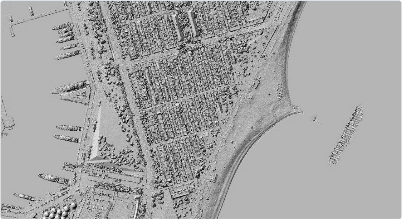
Figure 2. Digital surface model, hillshaded — the building front and harbour structures stand against the near-flat coastal plain.
